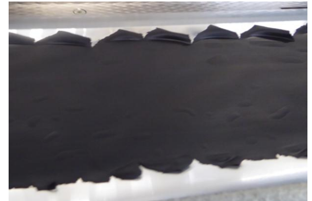
Example of a sample with poor edge quality
