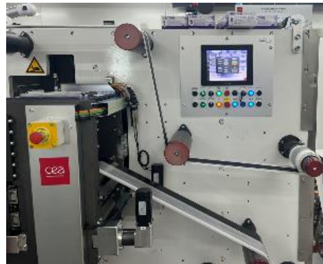
R2R co-lamination (multicomplexor)
