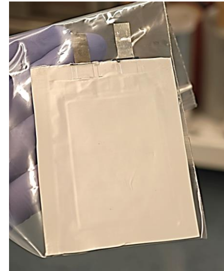
60 mAh jellified cell monolayer
