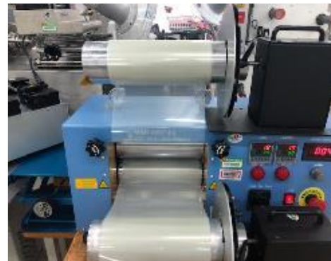
Lamination between two liners
